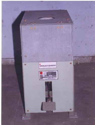
**Fig. 1** Photograph of the induction furnace used for casting of Al-SiC<sub>p</sub> composites
