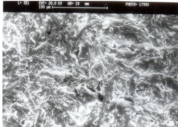
**Fig. 15** Scanning electron micrograph of gravity die cast pure aluminum sample at magnification 360X
