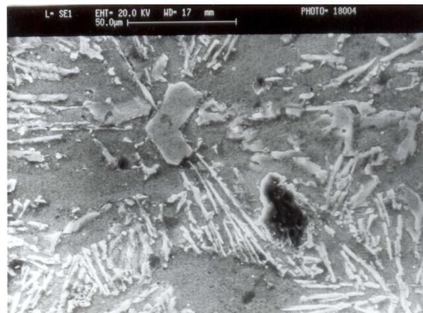
**Fig. 18** Scanning electron micrograph of gravity die cast Al-30 weight % SiC<sub>p</sub> composite sample at magnification 600X
