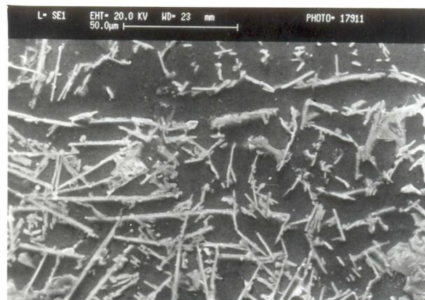
**Fig. 16** Scanning electron micrograph of gravity die cast Al-10 weight % SiC<sub>p</sub> composite sample at magnification 600X
