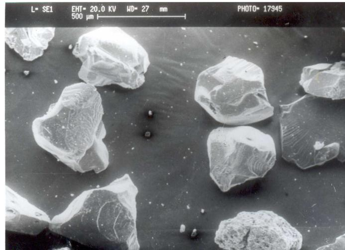
**Fig. 2** Scanning electron micrograph of SiC particulates used for casting of Al-SiC<sub>p</sub> composites
