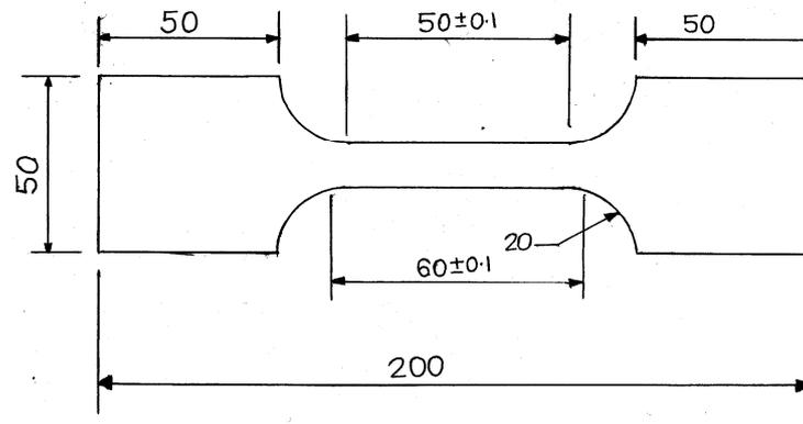
**Fig. 4** Specifications of the tensile test specimen
