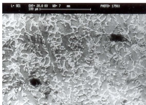
**Fig. 17** Scanning electron micrograph of gravity die cast Al-20 weight % SiC<sub>p</sub> composite sample at magnification 400X
