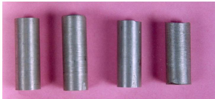
**Fig. 3** Photograph of the cast Al-SiC<sub>p</sub> composite specimens
