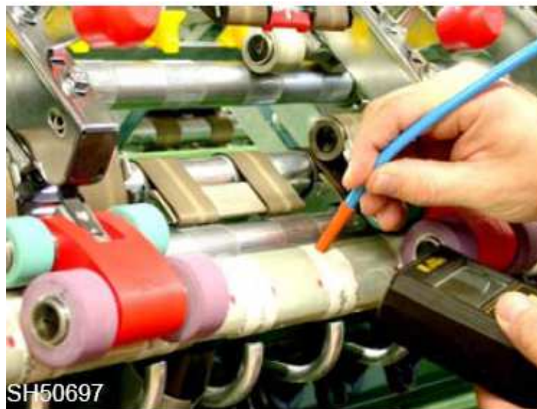
Figure 3 - Measurement of Negative Pressure
