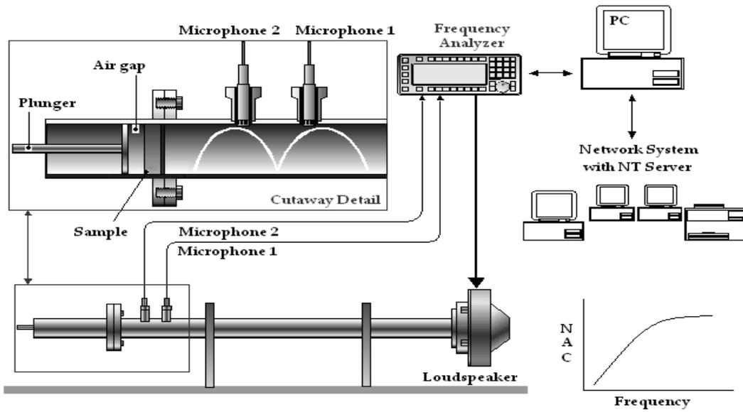
Figure 3: Impedance tube setup
