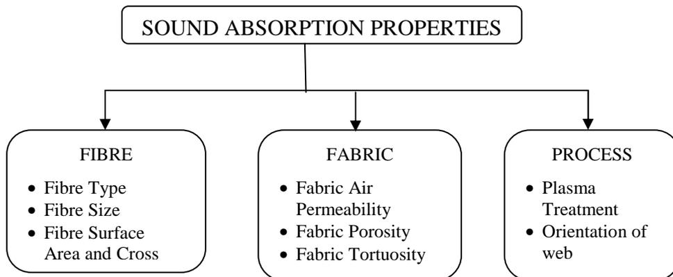
**Figure 7: Factors influencing sound absorption of nonwoven materials**
