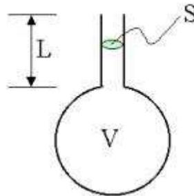
**Figure 5: Cavity resonator**
