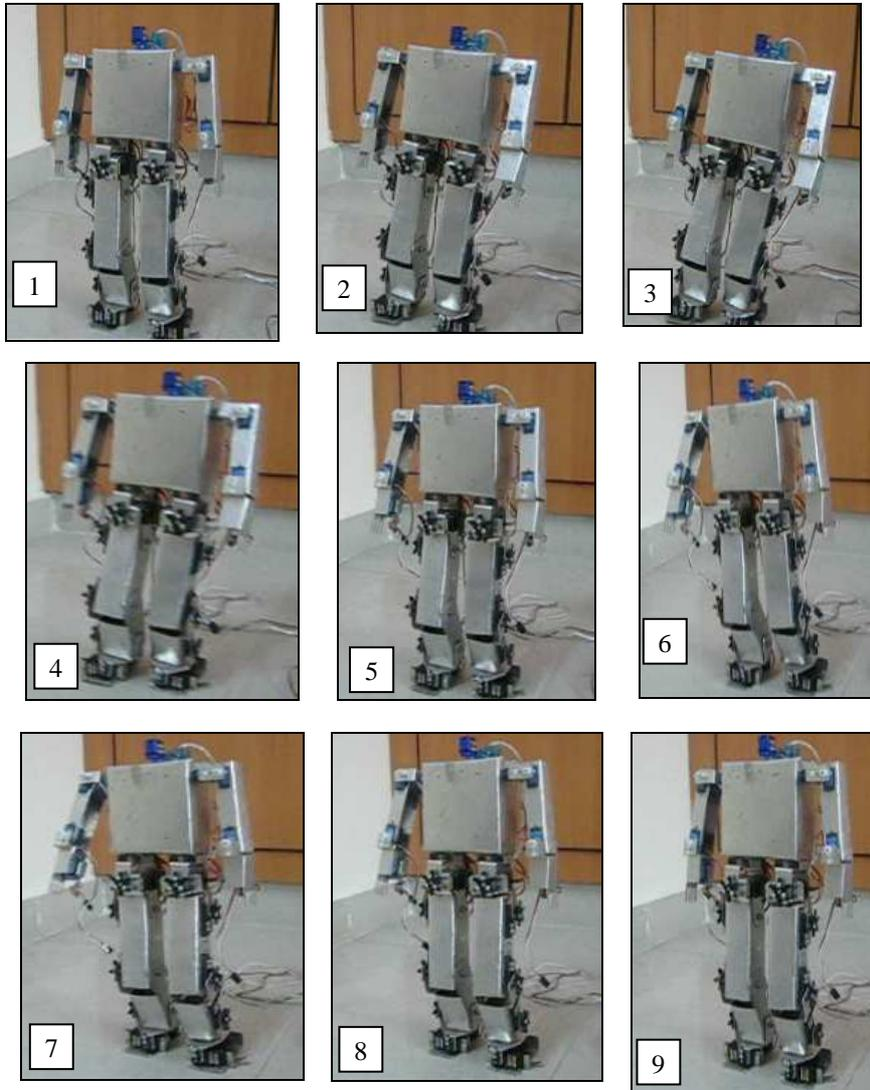
**Fig. 8** Sequence photographs of Robot walking on plain surface
