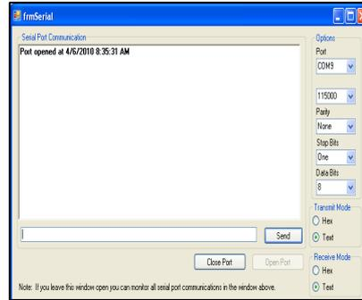
Fig. 6 Virtual COM port in a PC
