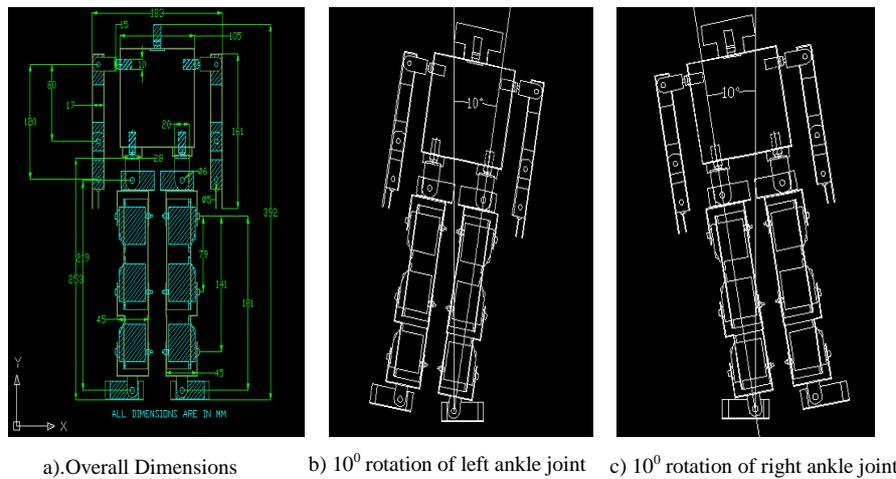
**Fig. 3 Auto-Cad Models of Human Robot (Gnano-369)**
