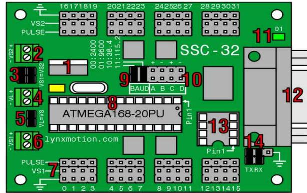
**Fig. 4 SSC-32 Servo controllers Board**
