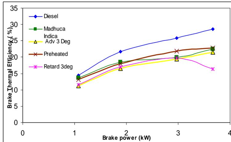
**Figure. 2 B TE of MI Oil with preheating and without preheating**
