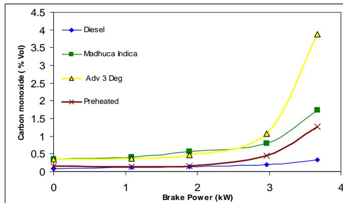
**Figure: 4 CO emission for MI Oil with and without preheating**
