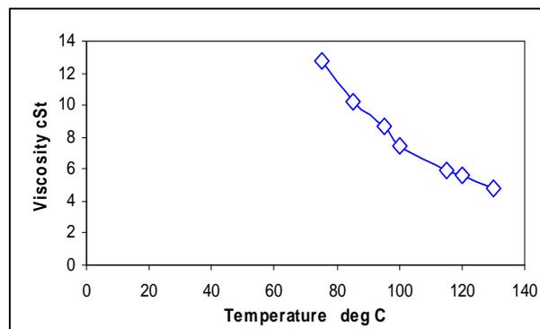
**Figure :1 Effect of temperature on Viscosity**
