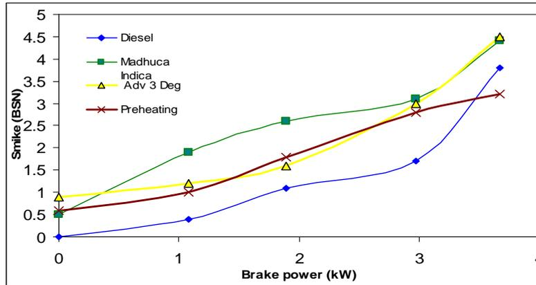
**Figure : 7 Smoke for MI Oil with/without preheating**
