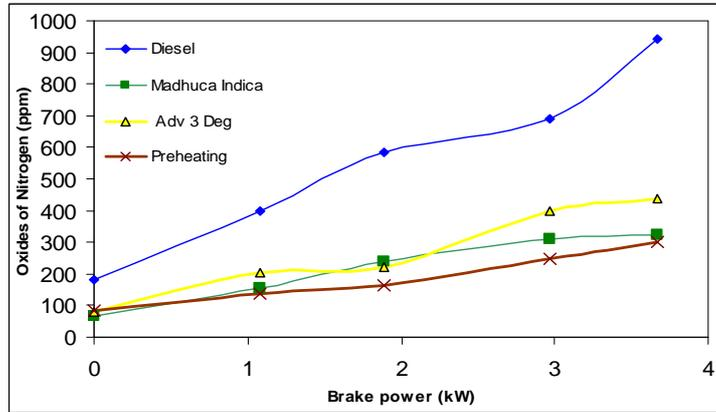
**Figure: 6 NO<sub>x</sub> for MI Oil with/without preheating**
