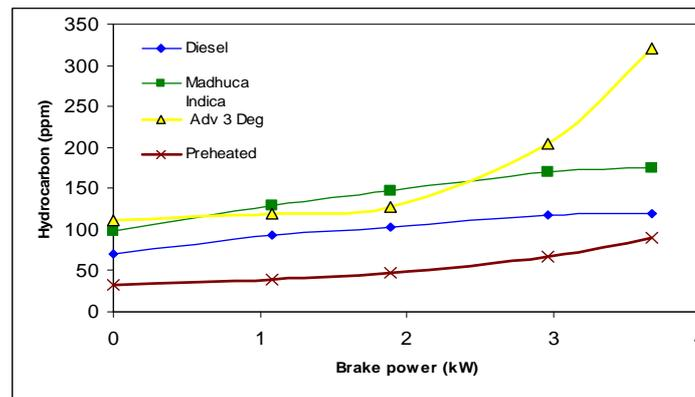
**Figure: 5 HC emissions for MI Oil with and without preheating**
