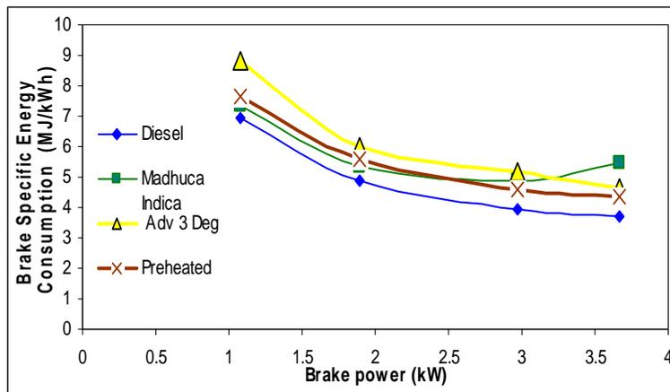
**Figure : 3 BSEC (MJ/KWh) for MI Oil with preheating and without preheating**
