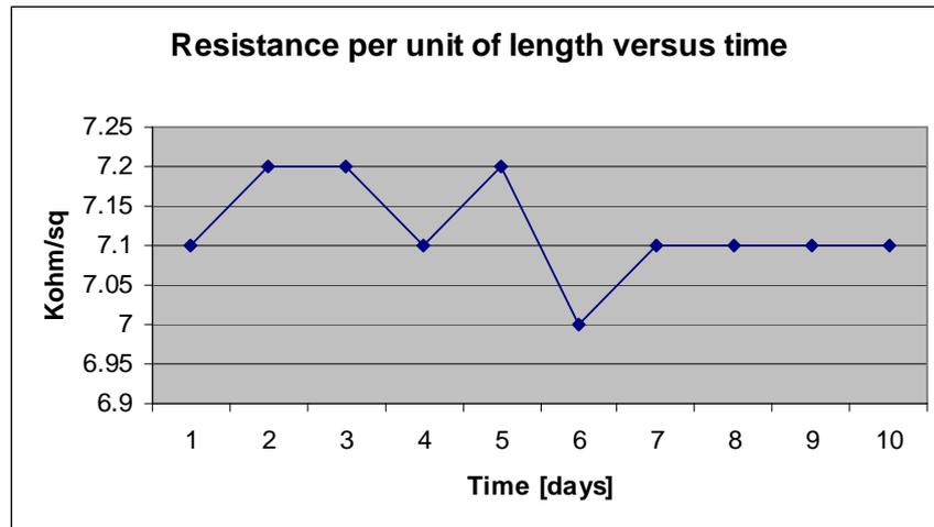
**Figure 2 : Resistance per unit of length versus time**
