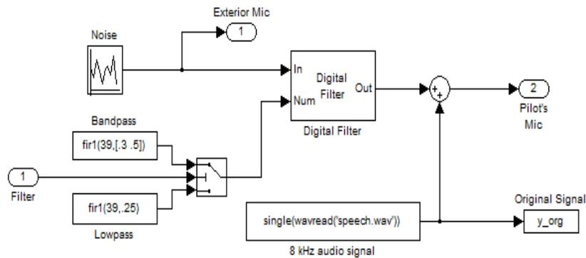
Figure (4) Internal Acoustic Environmental Simulink model
