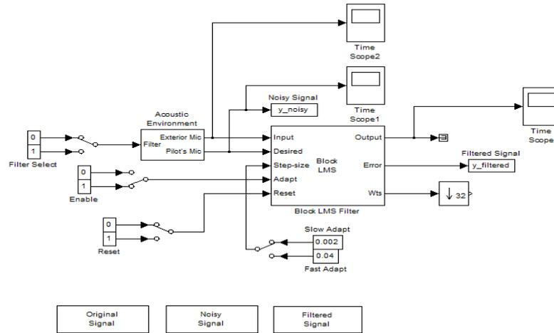
**Figure (5) Block LMS Simulink model**
