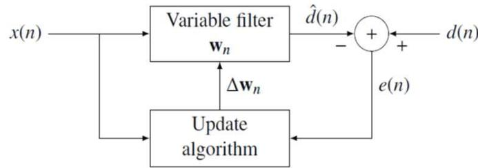
**Figure(1) General Block Diagram for Adaptive Filter**
