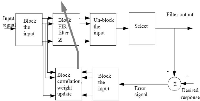
**Figure(3) : Block diagram of Block LMS algorithm**
