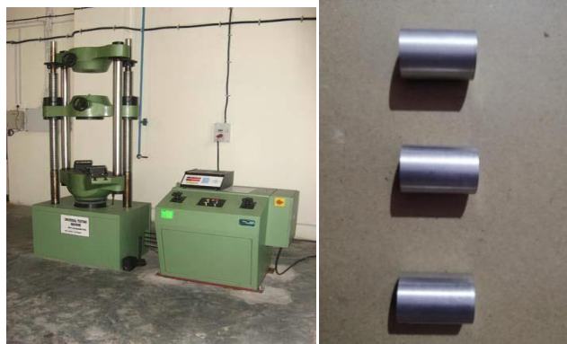
Figure 5.3: Compression Testing Equipment Testing Specimen
