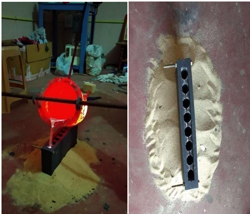
Figure 3.1.1: Pouring Molten Composites
