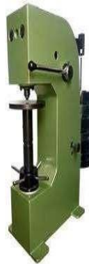
Figure 5.2: Brinell Hardness Testing Device Testing Specimen After Testing Specimen
