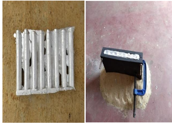
Figure 3.1.2: Casted Cylindrical Rods of ALTiO 2
