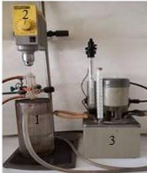
**1: Thermostatically-controlled Cell with a Jacket, 2: Stirrer with an adjustable Speed, 3: Thermostat
