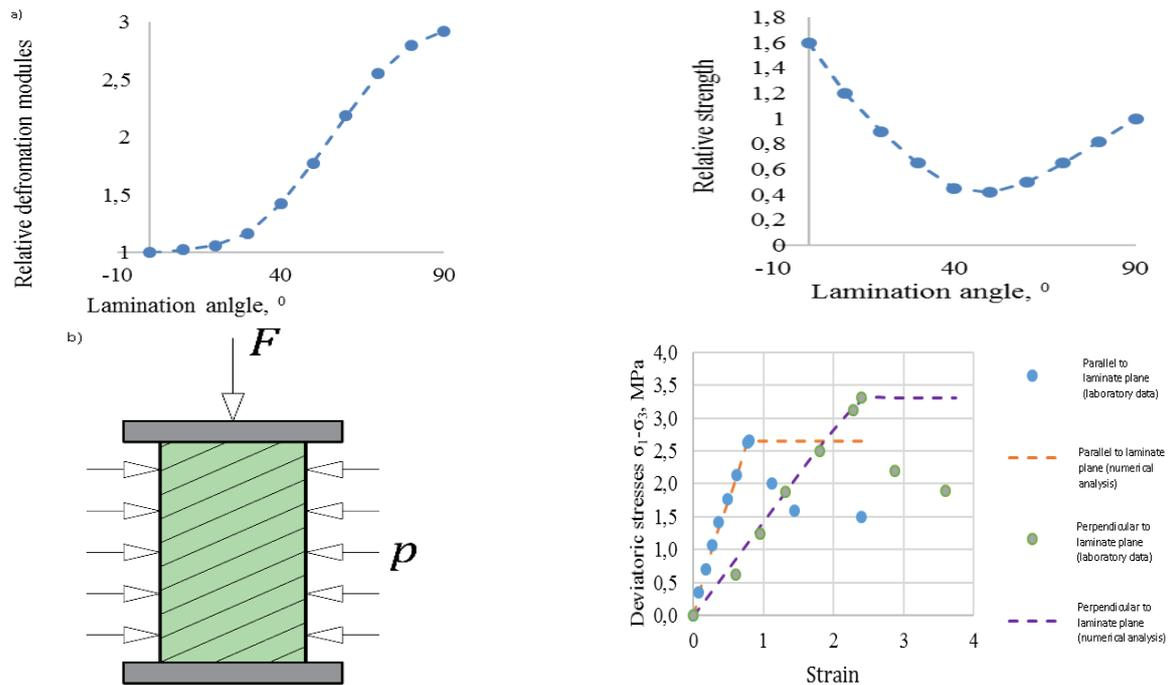
**Figure 2: Anisotropy of the Strength of Claystone-like Rocks: a - The Effect of Anisotropy on the Mechanical Characteristics of Rocks; b - Development of the Stress-Strain State of the Claystone-like Clay Rock.**
