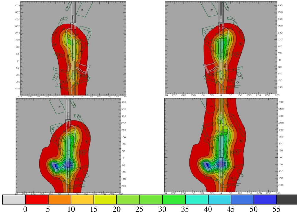
**Figure 4: Results of the Prediction of the Surface Deformations during the Construction of the Station Complex at Various Stages: a - Construction of the Workings of the Pit Bottom; b - Construction of a Secondary Traction Sub-Station and Adjoining Running Tunnels; c - Construction of the Left Station Tunnel; d - Construction of the Right Station Tunnel; e - Construction of a Complex of Workings of a Transfer Hub; f - After Completion of the Construction of all Underground Structures.**
