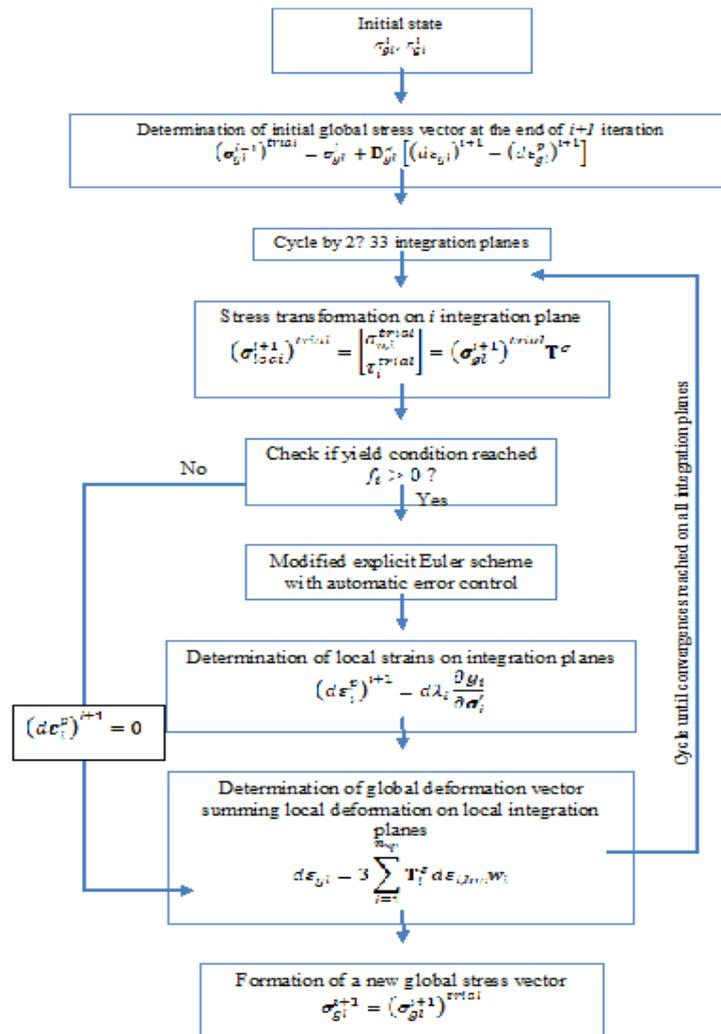
Figure 1: Algorithm for the Numerical Implementation of the Geomechanical Model in the Framework of the Multilaminar Environment Model.
