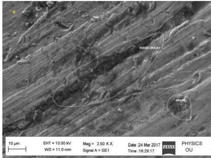
**Figure 4: Micro Structure of the Machined Sample at Experiment No 14, High Surface Finish**
