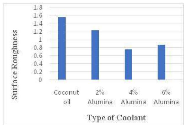
**Graph 2: Surface Finish vs Type of Coolant**
