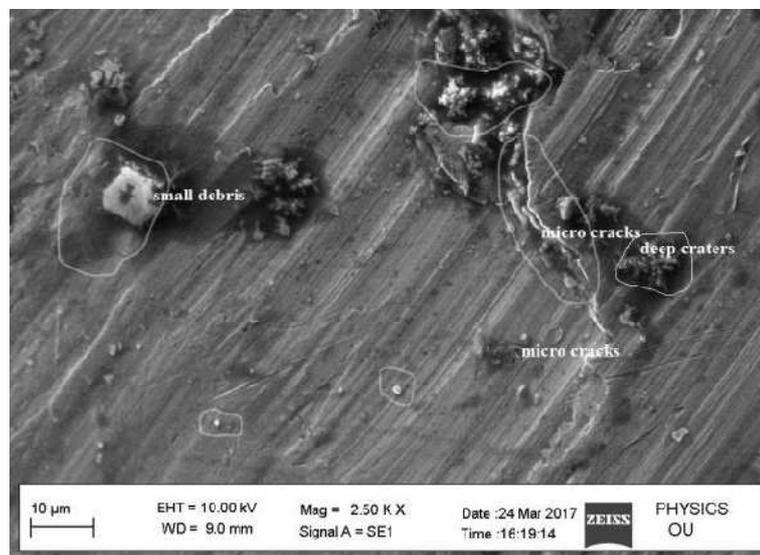
**Figure 3: Micro Structure of the Machined Sample at Experiment No 1, Low Surface Finish**
