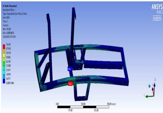
Figure 10: Equivalent Stress of Chassis
