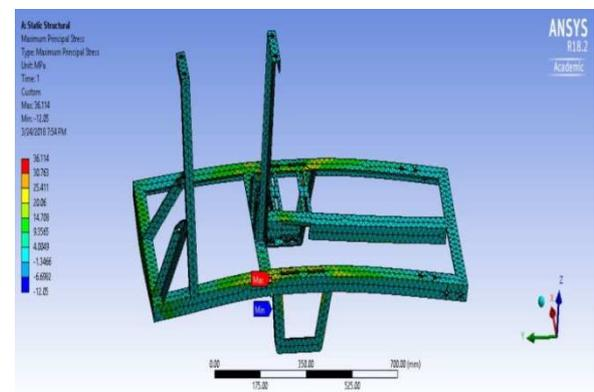
Figure 9: Maximum Principle Stress of Chassis
