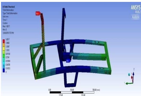
Figure 8: Total Deformation of Chassis
