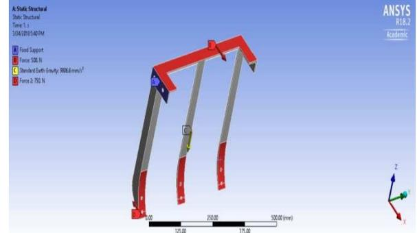
Figure 7: Boundary Conditions for Plough
