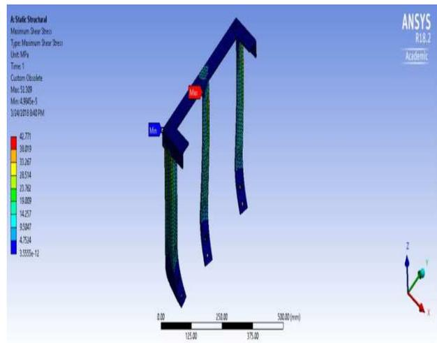
Figure 15: Maximum Shear Stress of Plough
