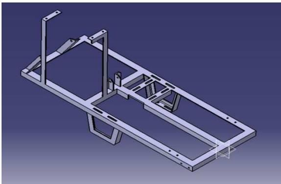
Figure 2: Chassis 3D Design for Power Tiller
