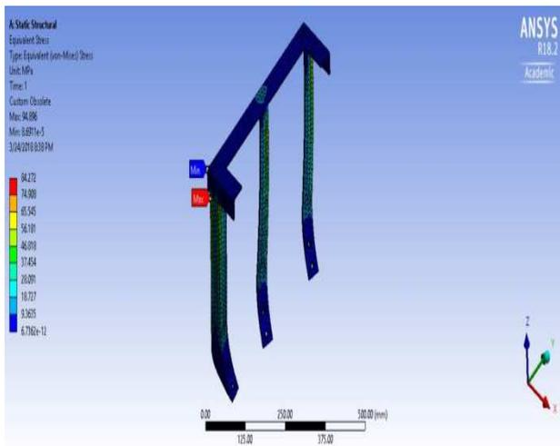
Figure 14: Equivalent Stress of Plough
