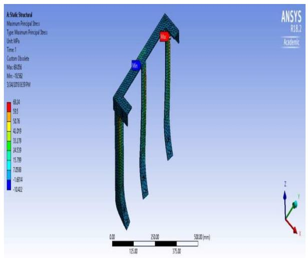
Figure 13: Maximum Principle Stress of Plough
