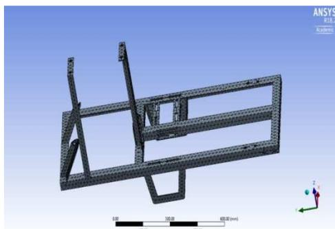
Figure 4: Meshing of Chassis
