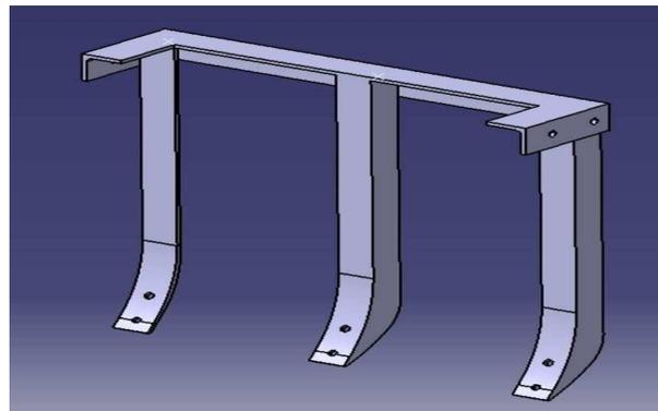
Figure 3: Plough 3D Design for Power Tiller
