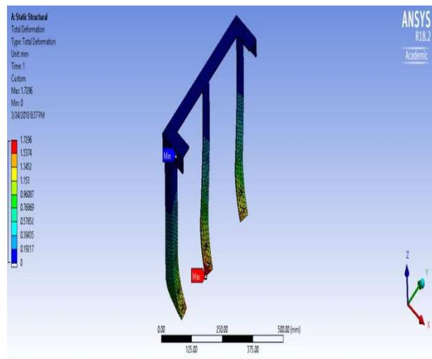
Figure 12: Total Deformation of Plough
