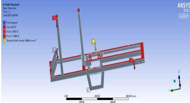
Figure 6: Boundary Conditions for Chassis
