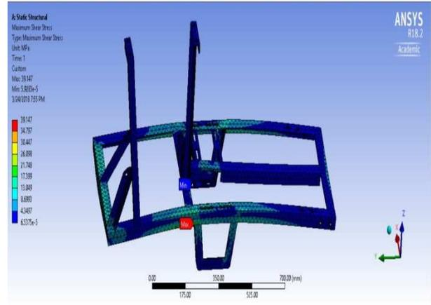
Figure 11: Maximum Shear Stress of Chassis
