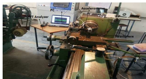
Figure 2: Actual Photo of Test Ring
