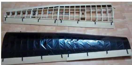
**Figure 6: Wing Covered with Film Cover**
