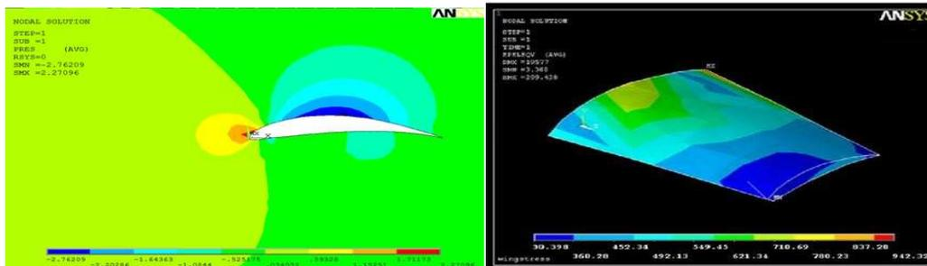
Figure 10: (a) CH10 (Smoothed) Airfoil Analysis (b) Wing Analysis
