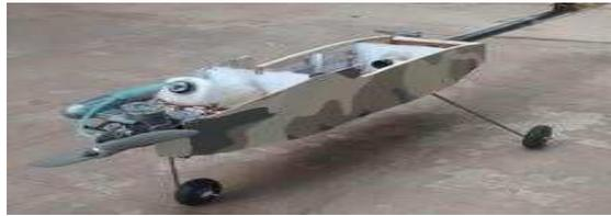
Figure 8: Side View of Fuselage with Engine Mount
