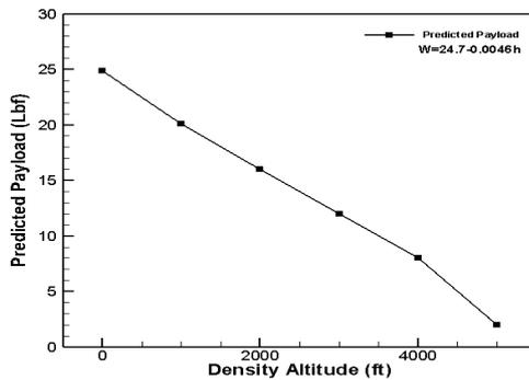
**Figure 11: Payload Prediction Graph**
