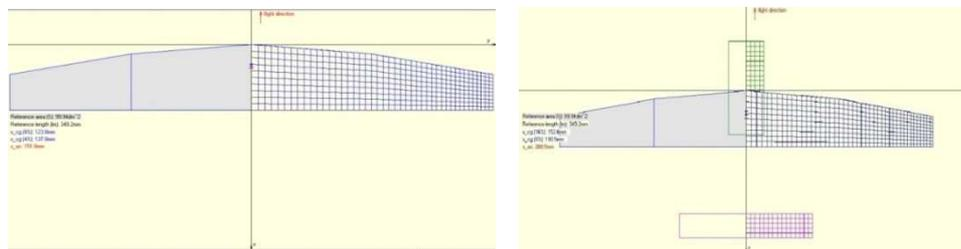
**Figure 13: (a) CG of the Wing (b) CG of the Aircraft**
