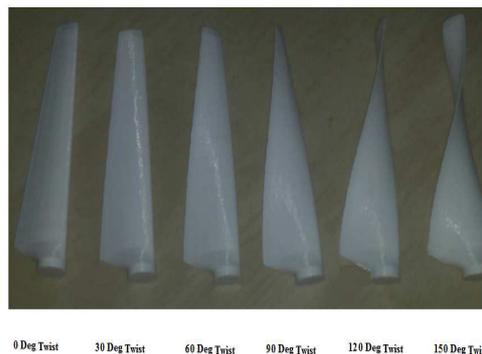
**Figure 5: Wind Turbine Blades with Various Twist Angles**
