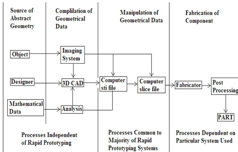
Figure 2: Main Process Stages Common to Most Rapid Prototyping Systems
