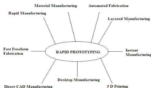
**Figure 1: Terminology Associated with Rapid Prototyping**
