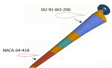
**Figure 3: Modified LM Blade**
