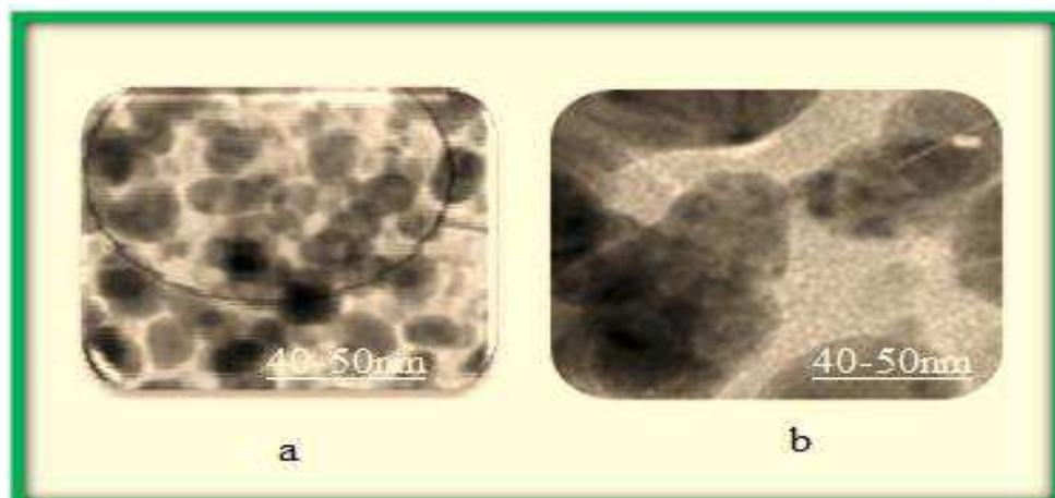
Figure 5: Transmission Electron Microscopy Images of Silver / *Moringa oleifera* after 24 Hours of Stirring
