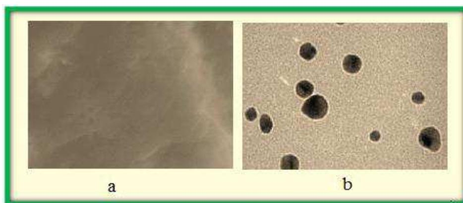
**Figure 6: Scanning Electron Microscopy Image of *Moringa oleifera* (A) and Silver/*Moringa oleifera* (B) Formation after 24 Hours of Stirring**
