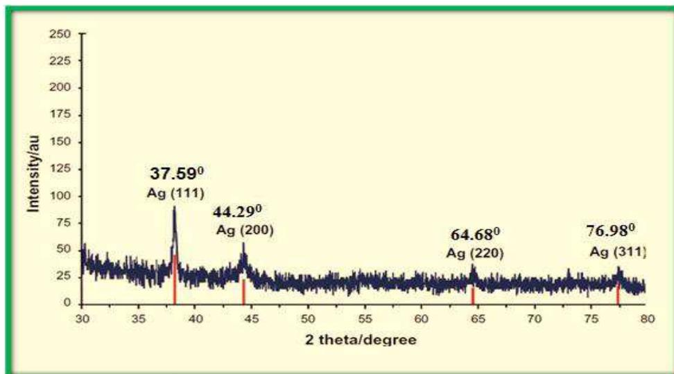
Figure 4: X-Ray Diffraction Patterns of Silver Nanoparticles (Ag-NPs) Synthesized in *Moringa oleifera* for Determination of Ag-NPs after 24 Hours of Stirring
