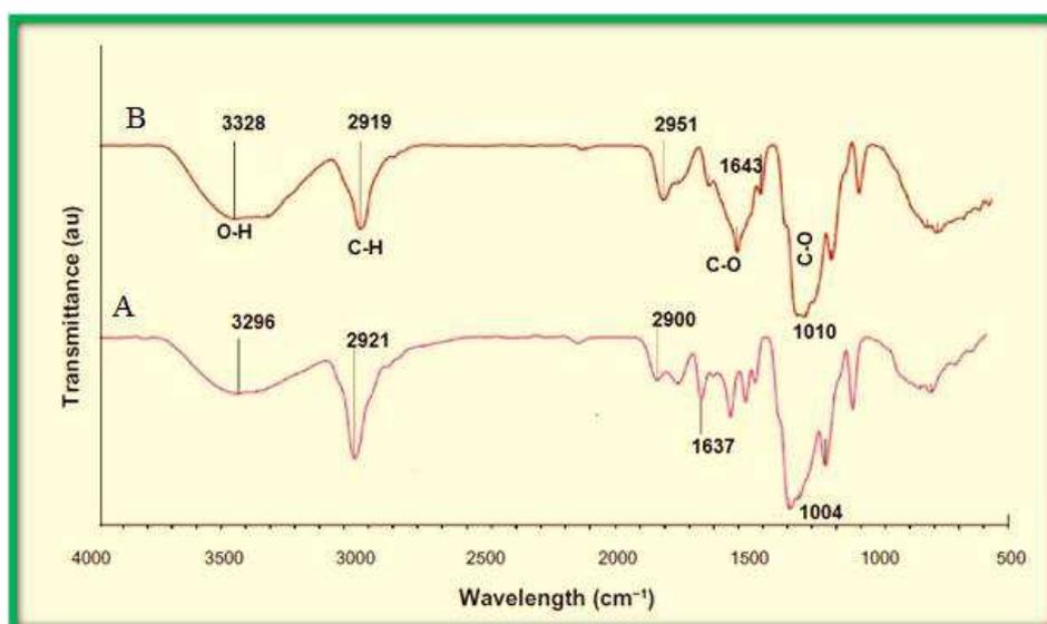
**Figure 7: Fourier-Transform Infrared Spectra for the *Moringa oleifera* Leaf Extract (A) and Ag/ *Moringa oleifera* (B) after 24 Hours from Biosynthesis Reaction**
