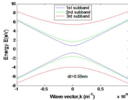
**Figure 3: The E(k) Dispersion Energy with CNT Sub-Band**
