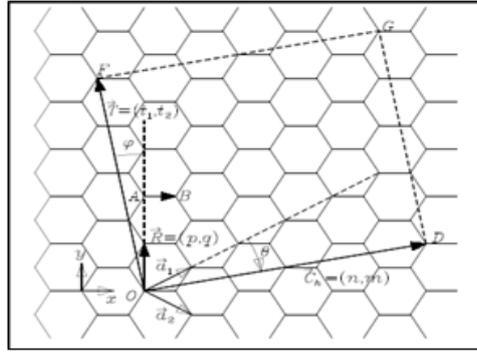
**Figure 1: Circumferential Vector  $\vec{C}_h$  and Vector  $\vec{T}$  in Real Space Graphene Lattice (Philipwong *et al*, 2011)**
