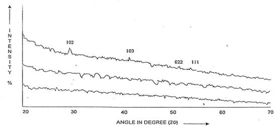
**Fig.1: X-Ray Diffraction Pattern of Cobalt Chloride Doped GaAs and Ge Multilayer Thin Film of Thickness 14nm Deposited at Different Substrate Temperature ( $T_s$ ): (a)  $T_s=273$  K (b)  $T_s= 300$ K and c  $T_s=350$  K**
