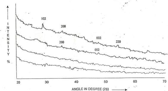
**Fig.2: X-Ray Diffraction Pattern of GaAs and Ge Multilayer Thin Film of Thickness 14nm Deposited at 300K, Annealed One Hour in Vacuum  $5 \times 10^{-5}$  torr at Different Temperature ( $T_s$ ): (a)  $T_s=373$  K (b)  $T_s= 473$ K and c  $T_s=573$  K**
