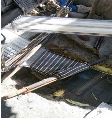
Figure 17: Pit Loom for Weaving
