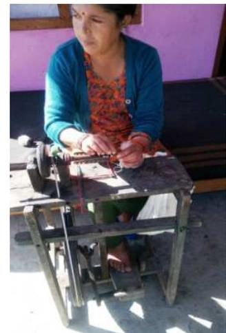
**Figure 9: Yarn Making using Spindles on Machine**
