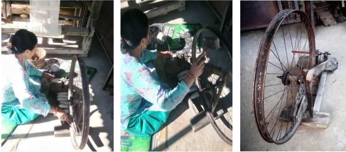
**Figure 12: Charka for Spinning**
