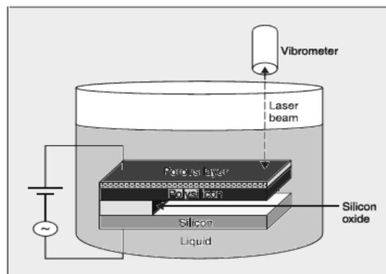
**Figure 5: A Triglyceride Biosensor with a Cantilever Beam in Liquid**
