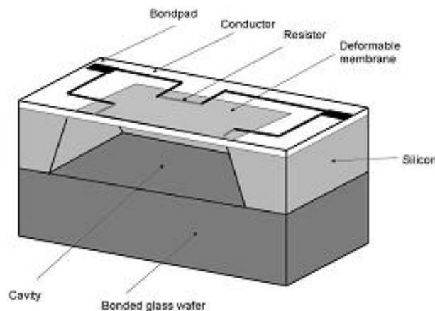
**Figure 4: Schematic Piezoresistive Pressure Sensor**
