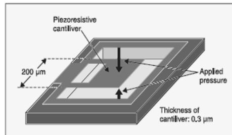
**Figure 15: MEMS Differential Pressure Sensor for an Insect-Like Ornithopter**
