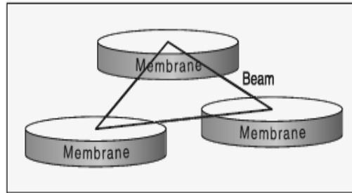
**Figure 10: Schematic Diagram of the Fly-Ear Inspired 2-D Sound Source Localization Sensor**
