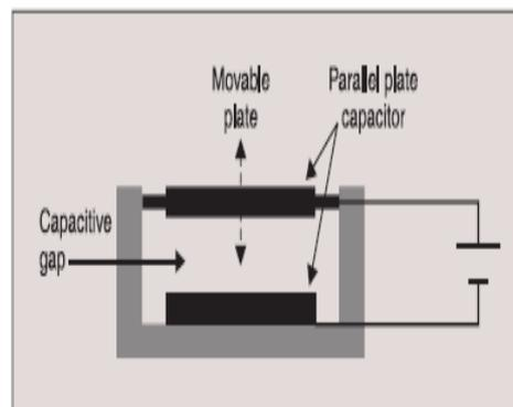
**Figure 20: Schematic Diagram of a Capacitor with one Movable Plate**
