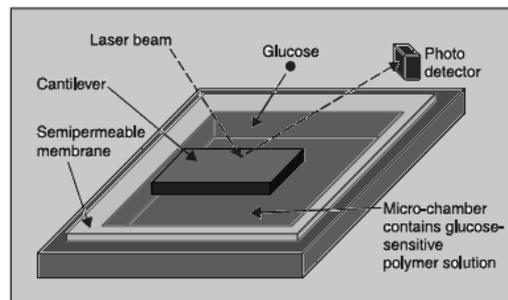
**Figure 7: A MEMS Affinity Sensor for Detection of Glucose**
