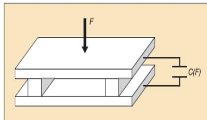
**Figure 13: Schematic Diagram of Tactile Capacitive Sensor**
