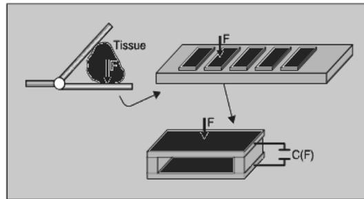
**Figure 8: MEMS Tactile Sensors for Quantifying Tissue Softness**
