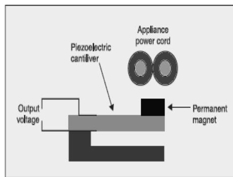
**Figure 19: Schematic of the Current Sensor**
