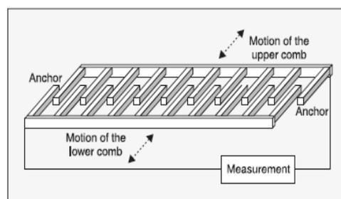
**Figure 12: Comb Drive or Finger Capacitive Design of Strain Sensor**
