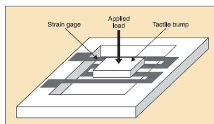
**Figure 14: Schematic Diagram of Tactile Sensor**
