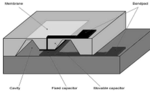
**Figure 3: Schematic Capacitive Pressure Sensor**
