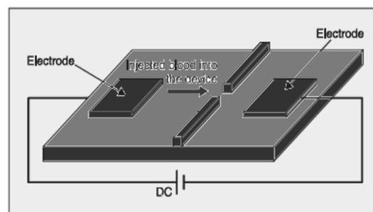
**Figure 9: Schematic Diagram of the Blood Counter Sensor**
