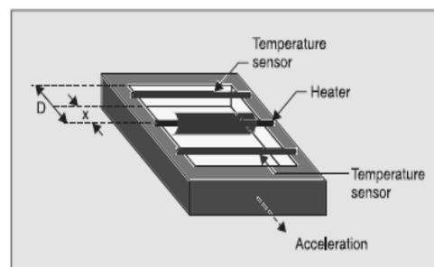
**Figure 11: Convective Acceleration Sensor**
