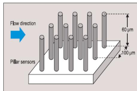
**Figure 18: Micro-Pillar Shear Stress Sensor**
