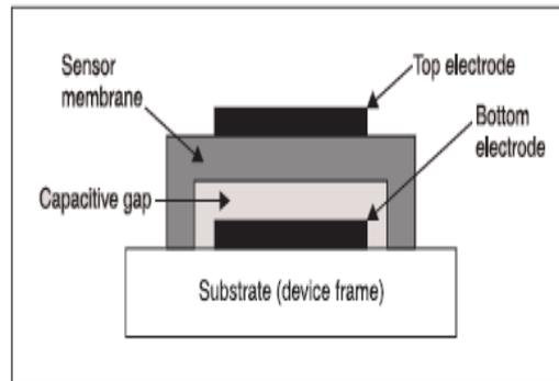
**Figure 16: Capacitive Transducer for Intramuscular Pressure Measurement**
