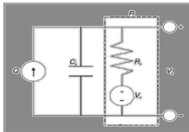
Figure 2: Equivalent Circuit for a Piezoelectric Micro Sensor
