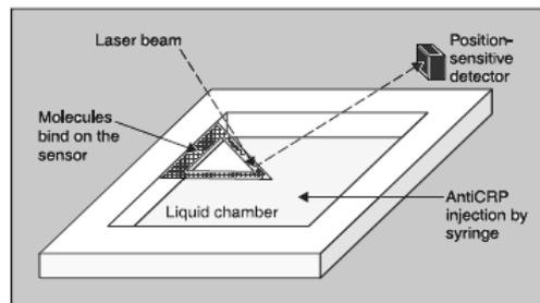
**Figure 6: Schematic Diagram of Bio-MEMS Sensor for CRP Detection**
