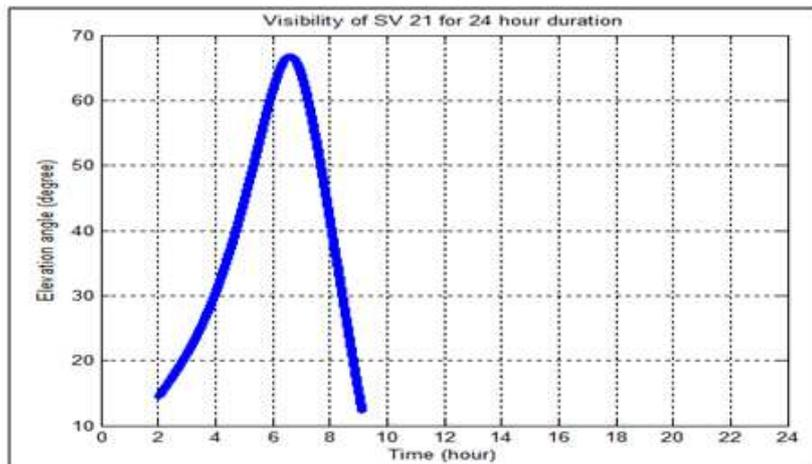
Figure 7: Visibility of Satellite Vehicle 21 for 24 Hours Duration
