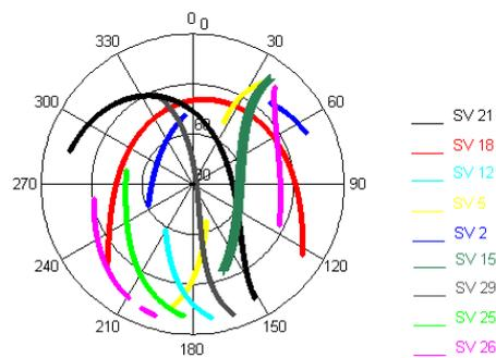
Figure 11: Polar Plot of Azimuth Angle Vs Elevation Angle of Nine Satellites
