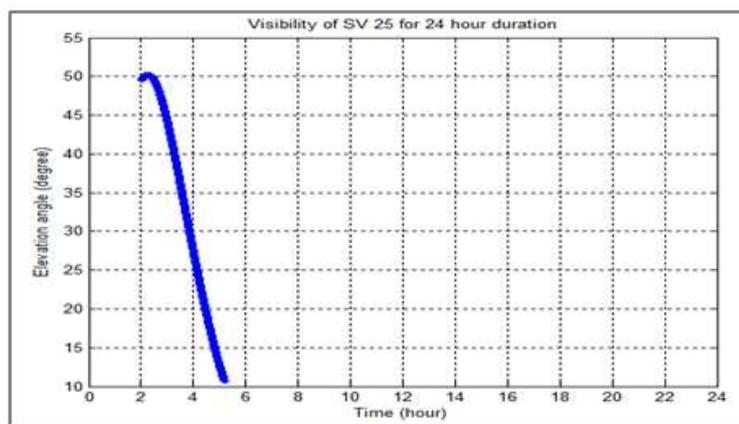
Figure 8: Visibility of Satellite Vehicle 25 for 24 Hours Duration
