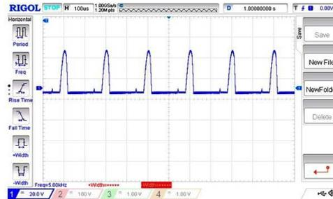
**Figure 17: The Typical View of the Voltage across the Primary of the Fly Back Converter Transformer**
