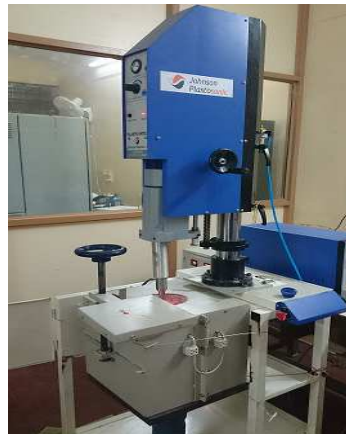
Figure 1: Ultrasonic Assisted Casting Machine Setup (NITW)
