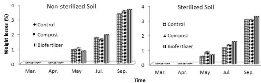
**Figure 5: Weight Loss (%) of Ecovio Tubes at Non-Sterilized and Sterilized Soil Treatments**
