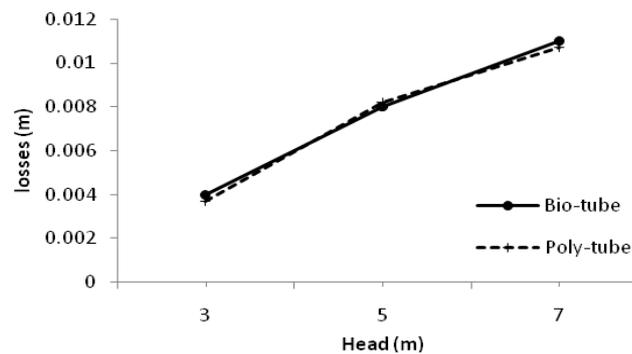
**Figure 6: The Friction Head Losses for Bio and Polytube**
