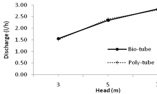
Figure 3: The Relationship between Pressure Head and Discharge
