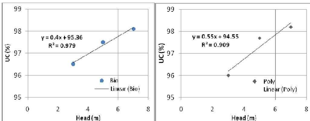
**Figure 5: Observed and Predicted UC vs Head for Bio and Polytubes**
