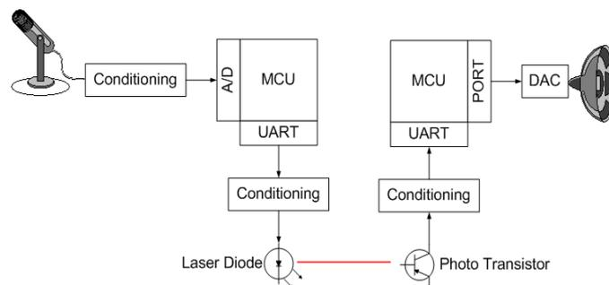
**Figure 5: Block Diagram of Laser Communication System**
