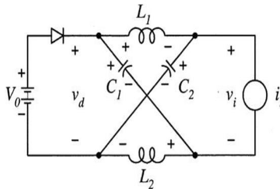
Fig.7: Equivalent Circuit of the ZSI Viewed from the Dc Link [9]
