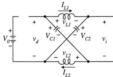
Fig.8: Equivalent Circuit of the ZSI Viewed from the dc dc Link When the Inverter Bridge is in the Shoot-Through Zero State
