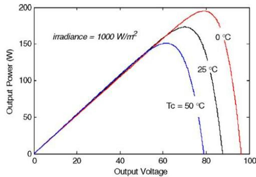
Figure 5: P-V Characteristic Curves of the PV Model at Different Operating Temperatures[6]
