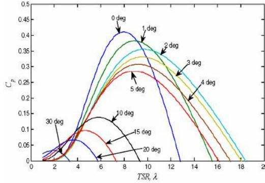
Figure 2: Cp - λ Curves of the WECS at Different Pitch Angles (Θ)[6]
