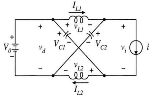
**Fig.9: Equivalent Circuit of the ZSI Viewed from the Link when the Inverter Bridge is in One of the Eight Nonshoot-Through Switching States [9]**
