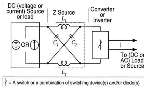
Fig. 6: General Structure of the Z-Source Converter [9]
