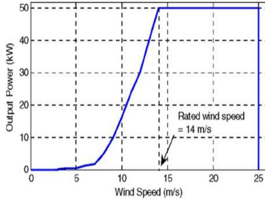
Figure 3: Output Power Vs. wind Speed[6]
