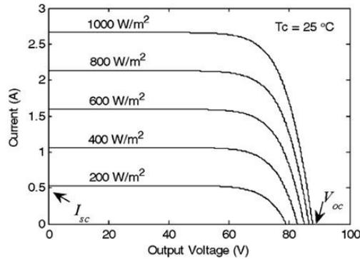
Figure 4: I-V Characteristics of the PV Model at Different Irradiances [6]
